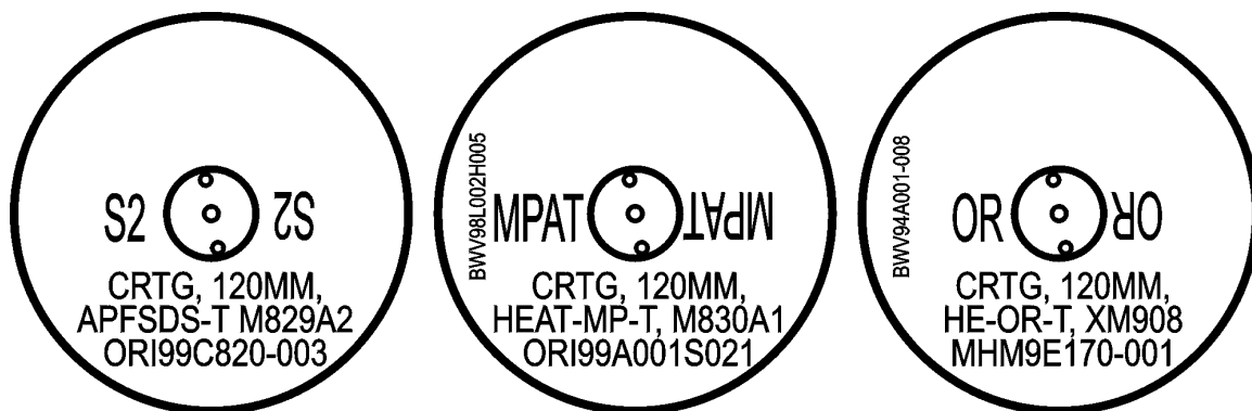
Figure 4-3. Aftcap Round-Type Quick Reference Markings.
